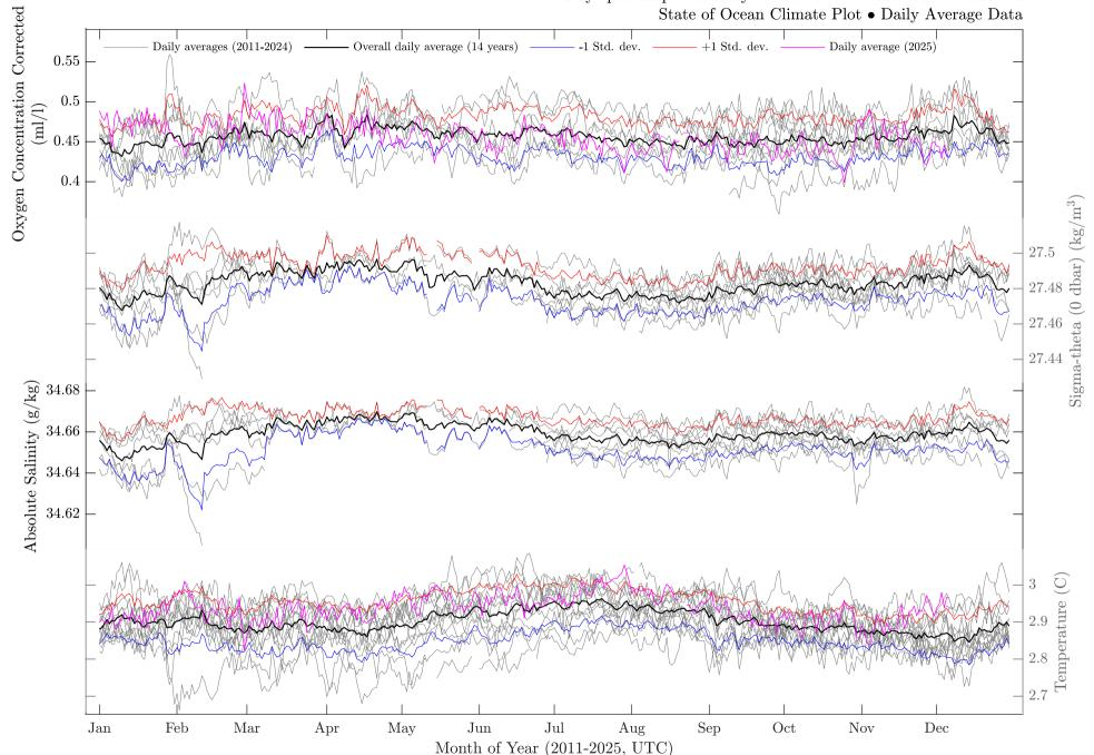
Sample period: 2.1 minutes (average). Comments: Clean Data (major quality failures (QAQC 3,4,6) excluded): all data plotted pass QAQC. QAQC testing complete, manual QAQC screening may be needed for recent data. See documentation for details. Standard deviations calculated from daily averages. Leap days excluded.
