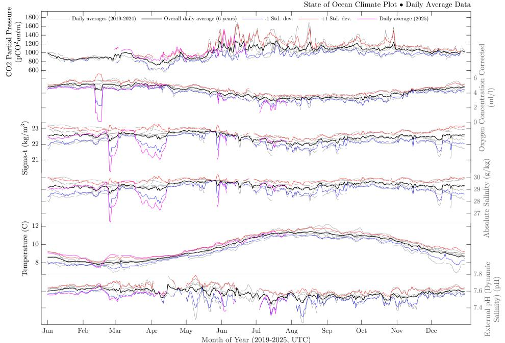
Sample period: 2.3 seconds (average). Comments: Clean Data (major quality failures (QAQC 3,4,6) excluded): all data plotted pass QAQC. QAQC testing complete, manual QAQC screening may be needed for recent data. See documentation for details. Standard deviations calculated from daily averages. Leap days excluded.
