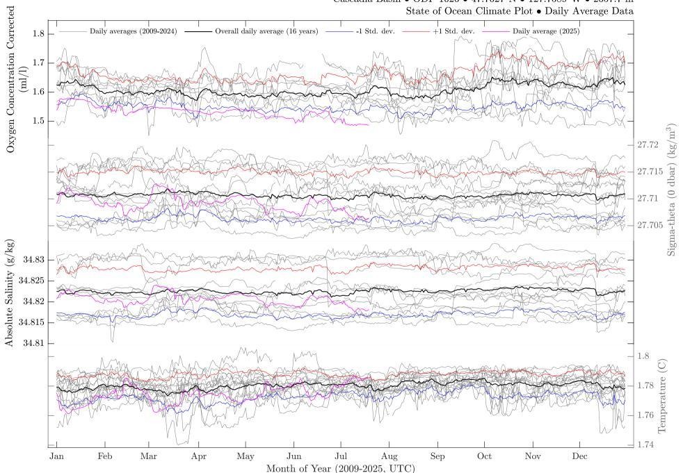
Sample period: 32.5 seconds (average). Comments: Clean Data (major quality failures (QAQC 3,4,6) excluded): all data plotted pass QAQC. QAQC testing complete, manual QAQC screening may be needed for recent data. See documentation for details. Standard deviations calculated from daily averages. Leap days excluded.
