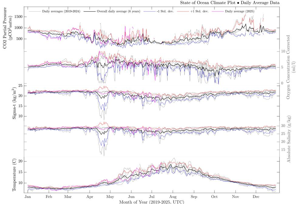
Sample period: 1 second (average). Comments: Clean Data (major quality failures (QAQC 3,4,6) excluded): all data plotted pass QAQC. QAQC testing complete, manual QAQC screening may be needed for recent data. See documentation for details. Standard deviations calculated from daily averages. Leap days excluded.
