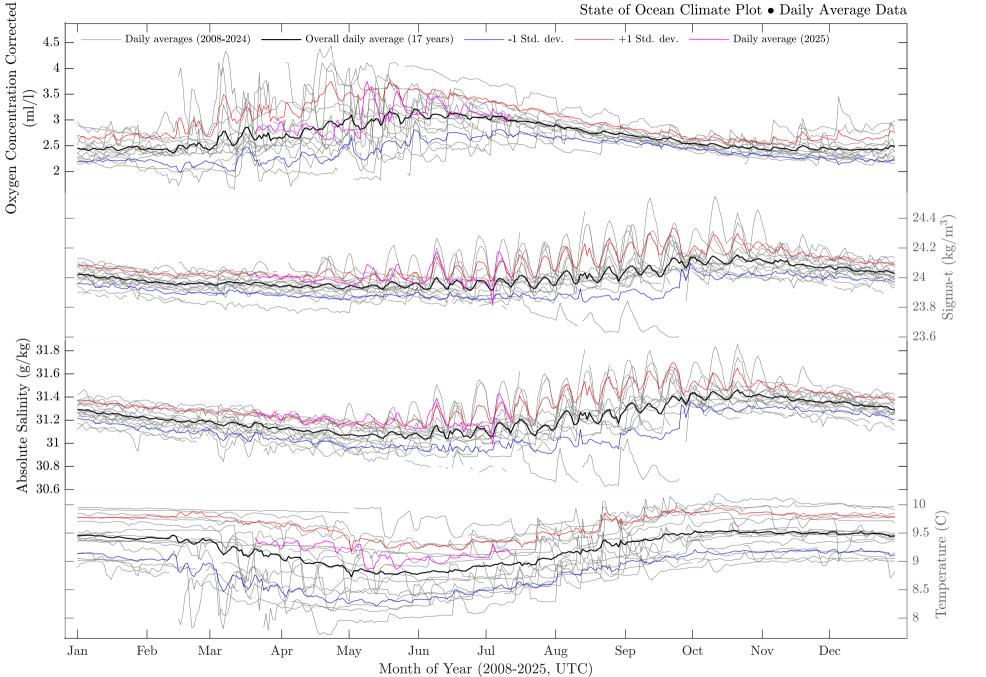
Sample period: 14.8 minutes (average). Comments: Clean Data (major quality failures (QAQC 3,4,6) excluded): all data plotted pass QAQC. QAQC testing complete, manual QAQC screening may be needed for recent data. See documentation for details. Standard deviations calculated from daily averages. Leap days excluded.
