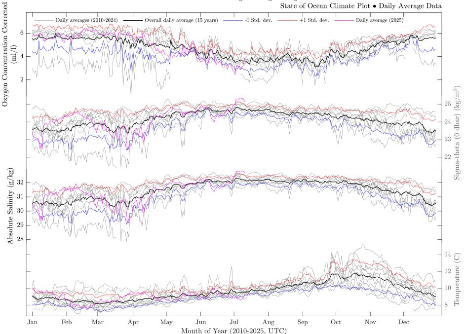
Sample period: 4.4 seconds (average). Comments: Clean Data (major quality failures (QAQC 3,4,6) excluded): all data plotted pass QAQC. QAQC testing complete, manual QAQC screening may be needed for recent data. See documentation for details. Standard deviations calculated from daily averages. Leap days excluded.
