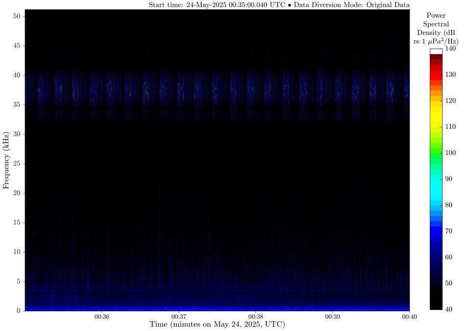
Comments: 34.1 % of spectrogram is less than 40 dB. Hann window with 50% overlap, 12800 samples per FFT window, temporal resolution: 0.05 s, spectral resolution: 10.0 Hz. Sample rate: 128000 Hz. Calibration is applied to each frequency bin individually. Downsampled to 0.10 s, 30.0 Hz resolution.
